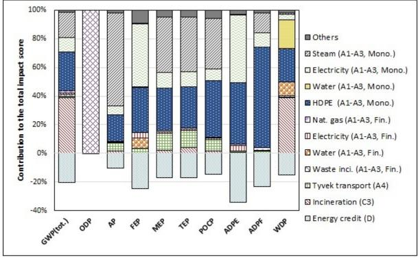
For most of the impact categories, more than 70 % of the impacts are dominated by the Tyvek® production (A1-A3) and in particular by the supply of HDPE granulates, steam and electricity.
