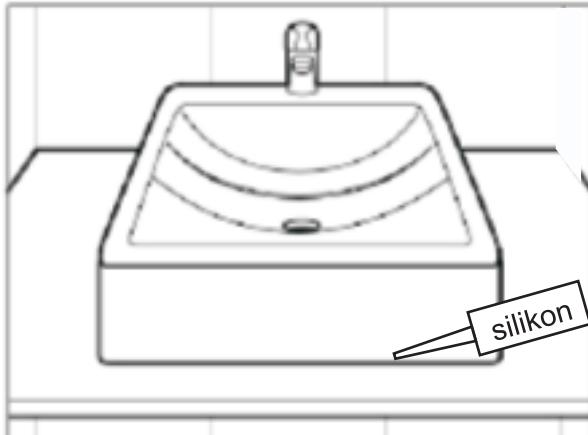
3. Washbasin is placed on the counter, tap is mounted on the washbasin, bottom edge of the basin is lined with silicone. For washbasin without overflow don't use close spout, stopper or clic clac armature, use full flow stopper! (in SIKO range - PZATKA).
