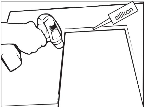
2. The counter is cut along the mark, lower surface of the counter is lined with silicone.
