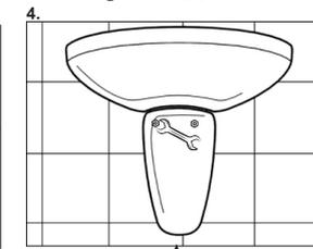
4. Semipedestal is placed on the bolts, nuts are tightened.
