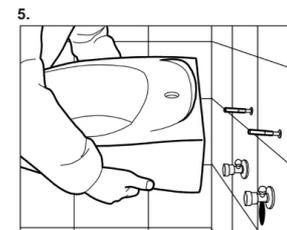
5. The washbasin is placed on the bolts, nuts are tightened.
