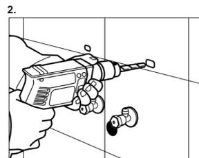
2. Washbasin mounting holes are marked on the wall.
