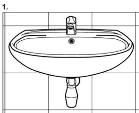
1. Basin should be installed in height of 85 – 88 cm from the floor.
