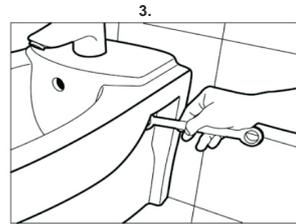
3. After the fixtures are connected to the bidet, bidet is installed in its place. Nuts are tightened.
