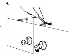
4. Mounting screw bolts are screwed into stops.
