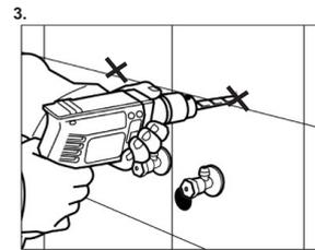
3. The marked places are drilled. Stop are placed.
