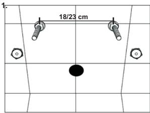
1. Concealed construction is assembled and prepared. Distance between screws for hanging the bidet can be 18 or 23 cm. In case change of wall hung bidet with another distance, please use the pattern 18/23 cm.
