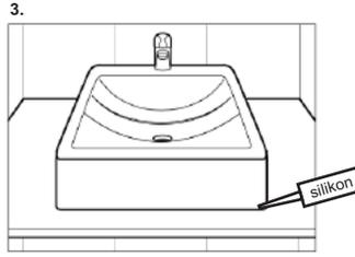
3. Washbasin is placed on the counter, tap is mounted on the washbasin, bottom edge of the basin is lined with silicone.
