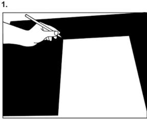
1. The products is placed on the counter to be used with the washbasin and the counter is marked.
