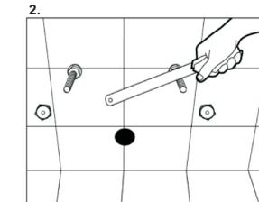
2. Bidet mounting screws are measured and cut to suitable length for mounting.
