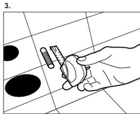
3. WC mounting screws are measured and cut to suitable length for mounting.
