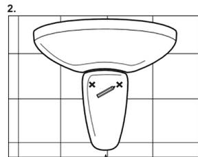
2. Semipedestal mounting holes are marked.
