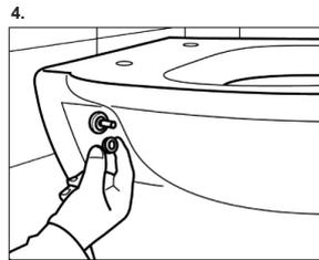
4. Wall-hung WC is put in place, mounted and nuts are tightened.
