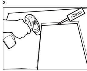
2. The counter is cut along the mark, lower surface of the counter is lined with silicone.
