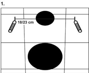
1. Concealed cistern is assembled and prepared. Distance between screws for hanging the toilet can be 18 or 23 cm. In case change of wall hung toilet with another distance, please use the pattern 18/23 cm.
